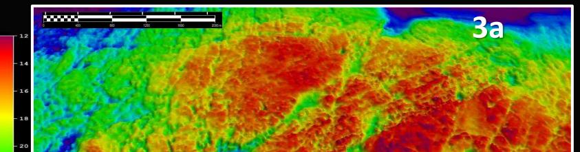
3a: Oblique view of study area Figure 3: 3D 5m (V.E.=2.7x) CUBE BASE Surface
